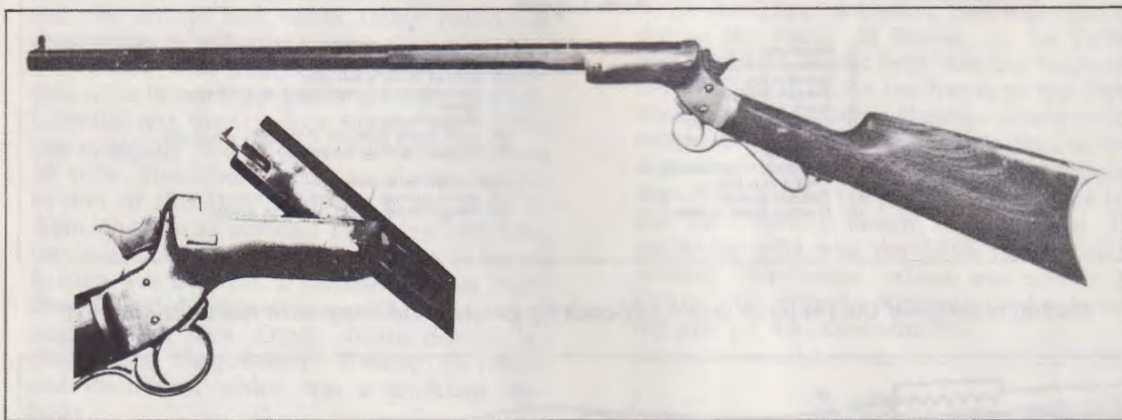
The first Stevens rifle used the tip-up action, a variation of the falling (dropping) block system.
