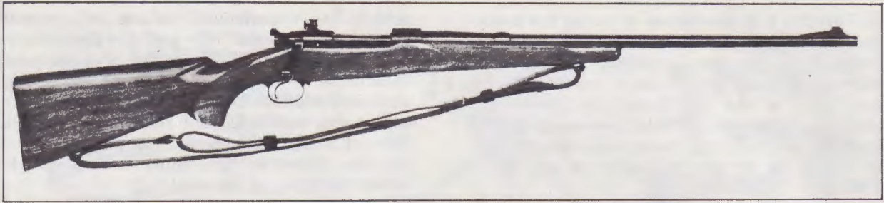
The Winchester Model 70, of turning-bolt design, was used for sporting and made the Winchester Arms Company famous.
