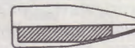
Hollow Point A popular varmint bullet with open tip and thin jacket. (Varmint bullets come also with lead points.)
