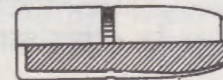
Flat Point A Round Nose variation used in rifles with tubular magazines.
