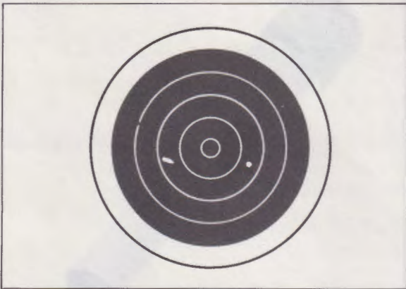
The KEYHOLE imprint at the left on the target shows that the bullet did not hit point on.
