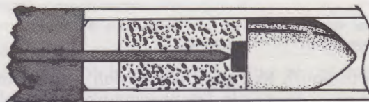
The long, thin firing pin of the NEEDLE GUN penetrates the base wad and powder to strike the cap.
