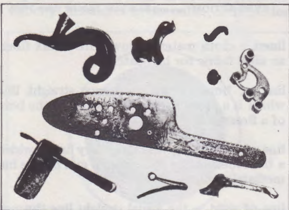
The nomenclature of this Scott LOCK, basically a percussion or breech-loading type, is, clockwise: hammer, tumbler, swivel, tumbler screw, bridle, sear, sear spring, and mainspring held in cramped position. In the center is the side plate, upon which the other parts are mounted.
