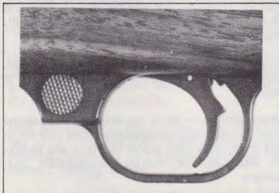
One of the most simple types of SAFETIES is this giant head, shown here on a .44 Ruger.
