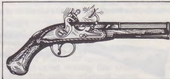
Original drawing of an early SNAPHAUNCE showing the ignition principle.
