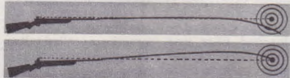
Sight adjustments must be made to ZERO the shots in the center of a target at various distances.
