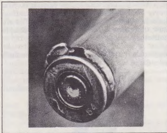
Reloaders must check used brass carefully to avoid loading a RUPTURED CASE such as the one above.
