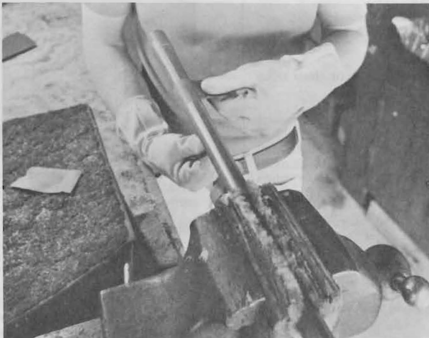
FIGURE 19 — Polishing goes fast when you use a padded vise.
