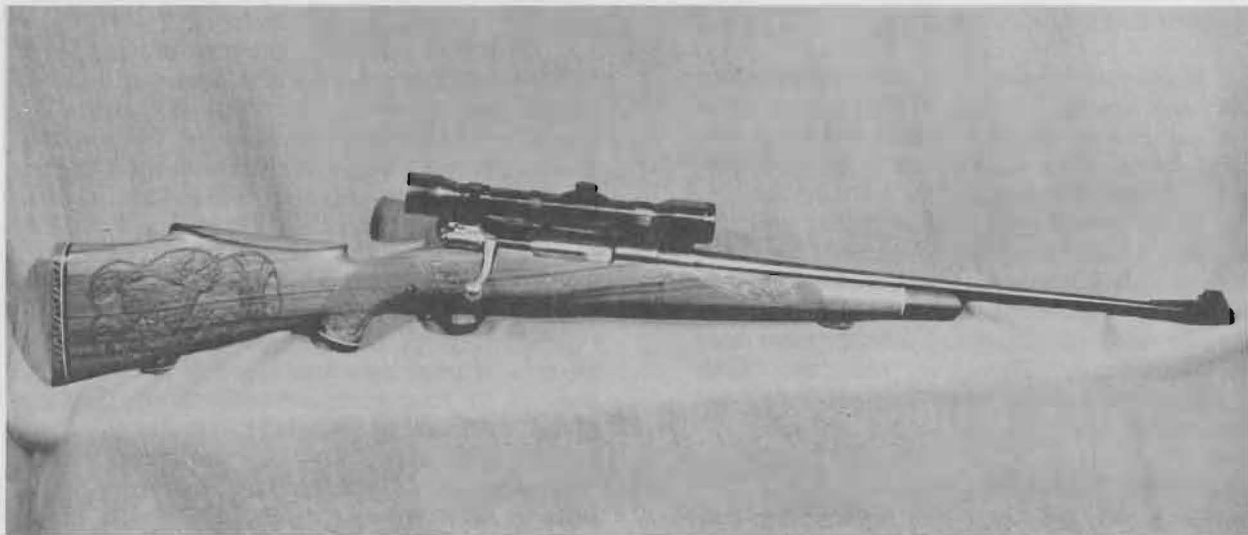
FIGURE 8 — Expensive custom sporters made before World War II and shortly thereafter, like the Mauser shown, were almost always blued by the “hot water” blueing process.
