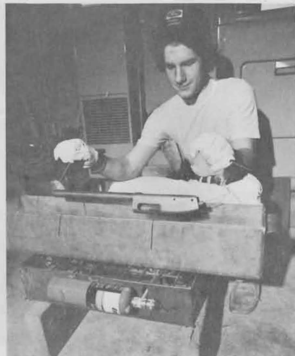
FIGURE 21 — Z-shaped handles are necessary for parts handling, even if you use plug handles for the barrel.
