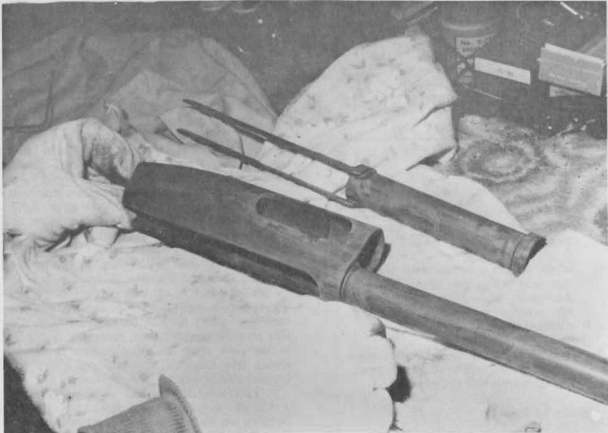
FIGURE 26 — Appearance of steel after blueing solution has "worked" about five minutes.
