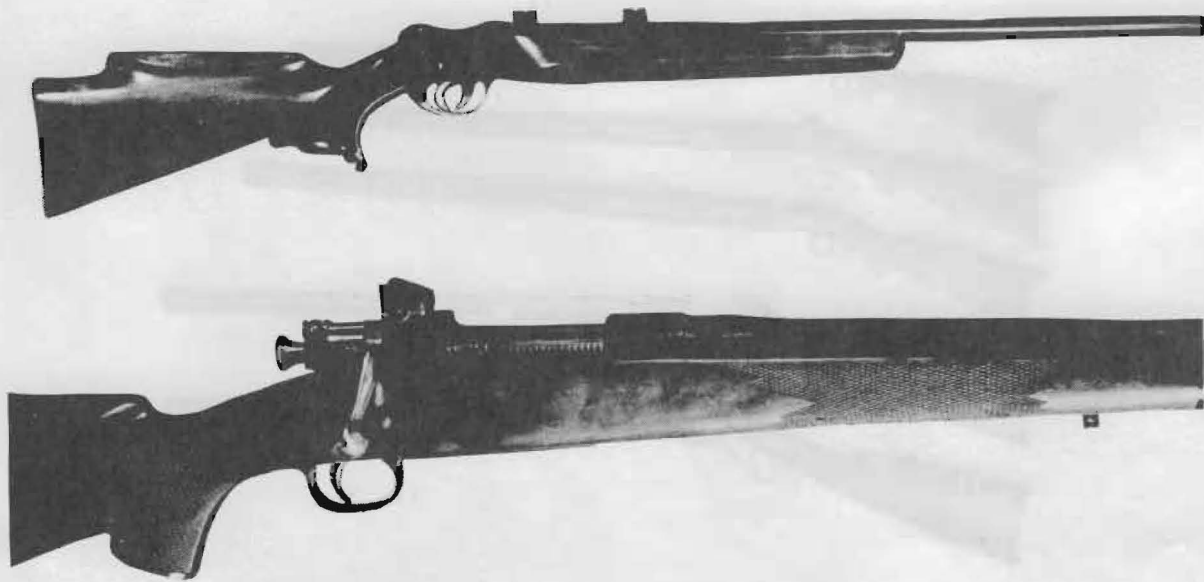
FIGURE 12 — Springfield rifles, released as surplus after World War I, were often sporterized and reblued by the "hot water" process.
