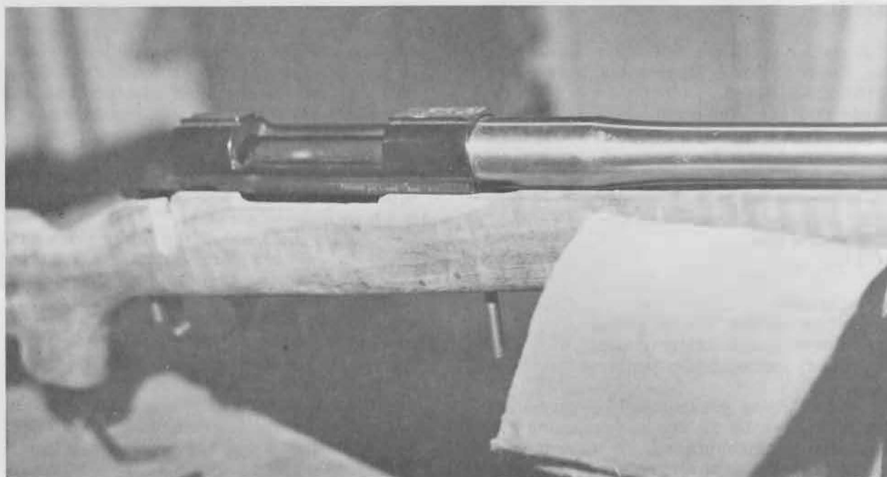
FIGURE 31 — "Hot water" blueing works well on new metal. Usually, receiver and action are blued simultaneously.
