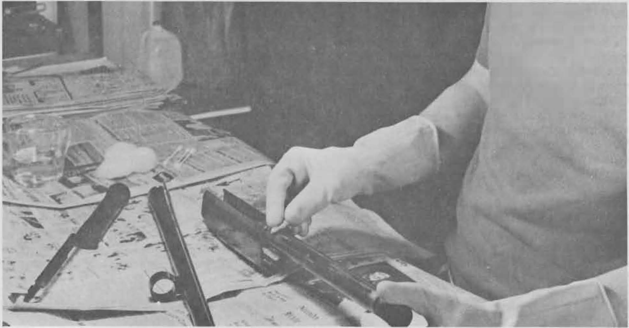
FIGURE 17 — Commercial removers or your “homemade” solution, quickly strip off the old finish.
