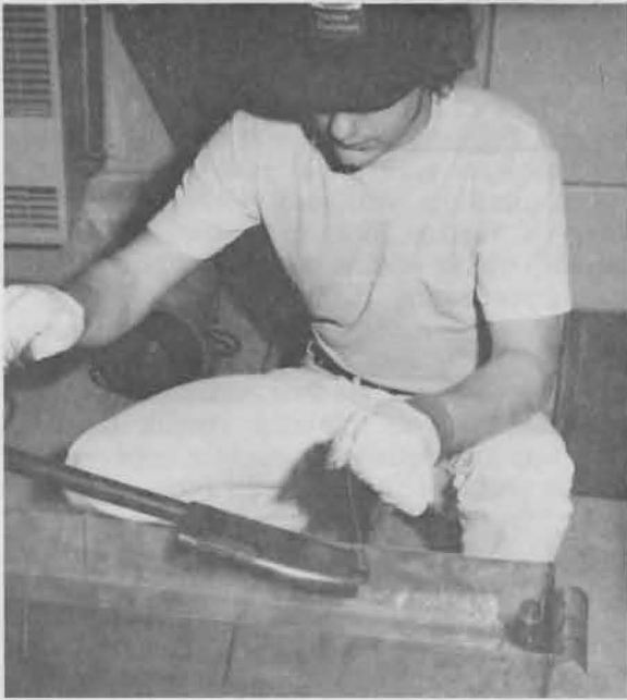
FIGURE 25 — Receiver ready for its first blueing solution application. Bottle (in corner) follows last part from tank.
