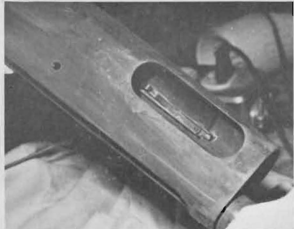
FIGURE 18 — The former blueing is replaced with a grayish film which is rinsed off with warm tap water.
