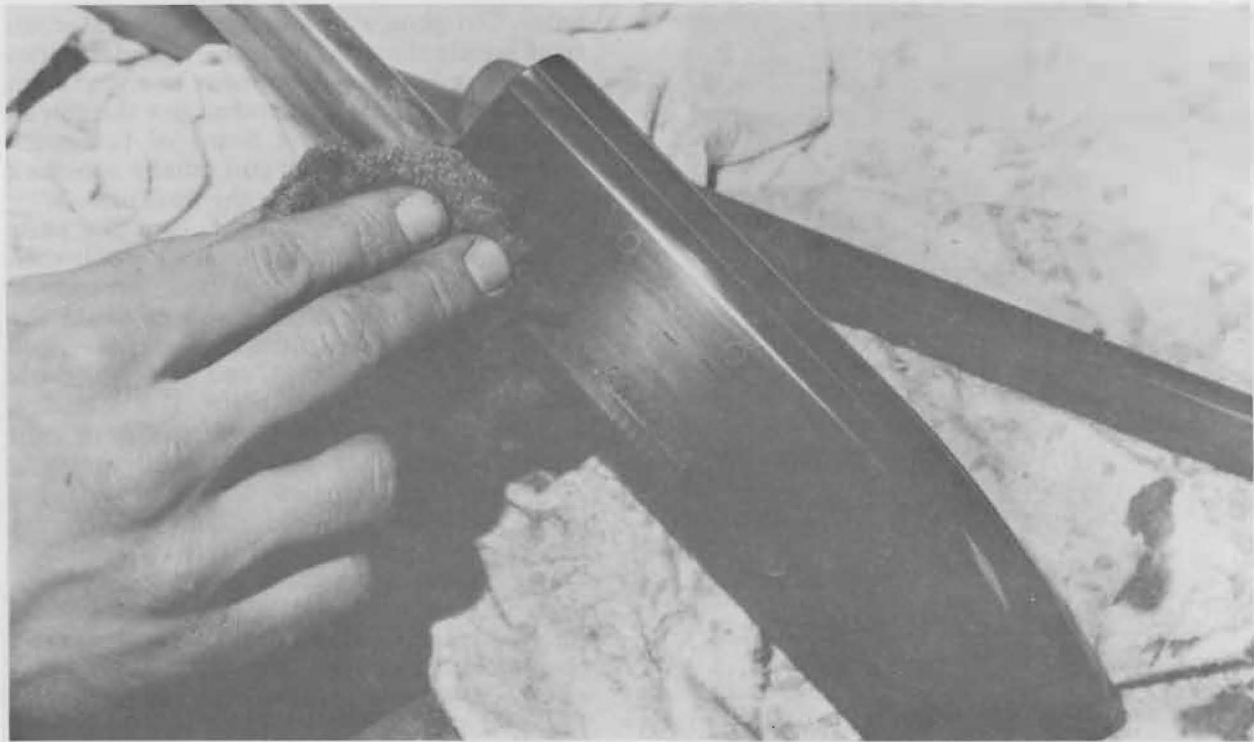
FIGURE 29 — Final carding with oil-saturated fine steel wool brings out that old-time satin finish.
