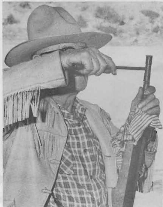
STEP 4 – Cover the muzzle with the patching material and start a round ball with the short starter. It is sometimes necessary to use a light hammer to seat a tight ball.
