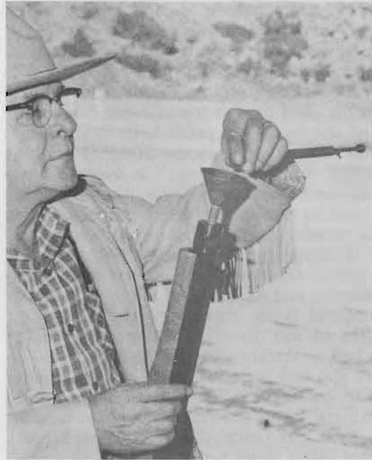
STEP 2 – Pour powder down the bore of the rifle, using a small funnel to prevent spillage.
