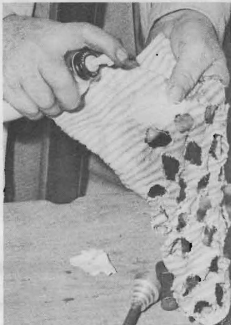
STEP 3 – Lubricate the patching material with a soluble oil solution or commercial lubricant.
