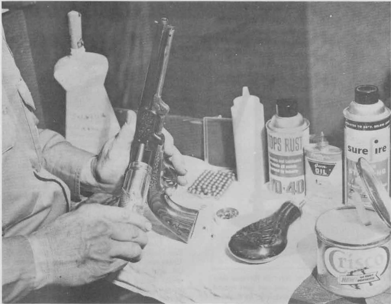
FIGURE 36 — The cap 'n' ball revolver is loaded using a powder flask with a metering tube to get the correct charge. Only one chamber at a time is loaded for safety and ease of handling. Powder is followed by round balls, covered with Crisco or other lubricant. Then the nipples are capped.
