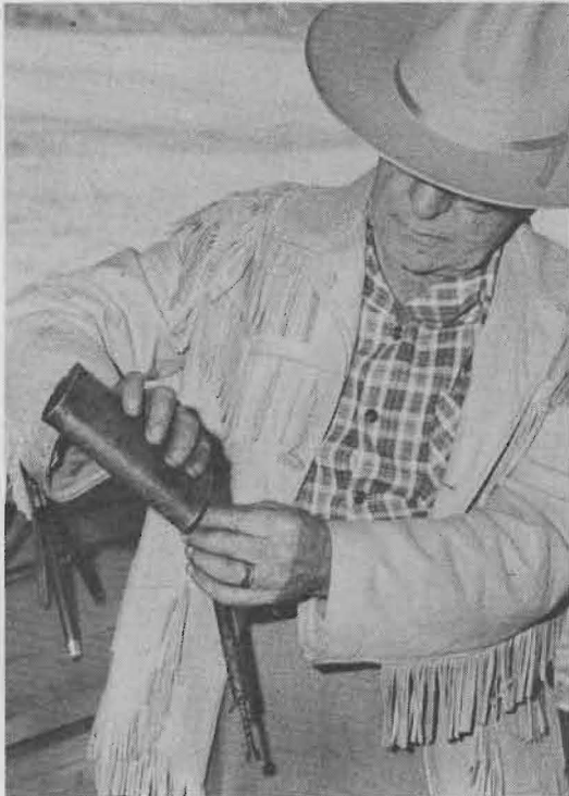
STEP 1 – Pour powder from a horn or other container into the powder measure.
