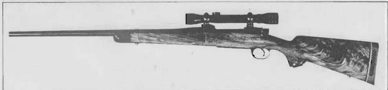
FIGURE 11 — Classic sporter with distinctive claro walnut stock. Note the trim lines and the swirls or flame in the butt.
