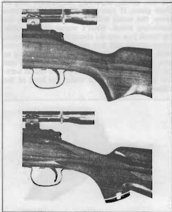
FIGURE 27 — A grip cap can greatly enhance the appearance of a pistol grip as shown by the reworked stock (bottom). The same stock (factory original) is at the top. (Photo courtesy NRA)
