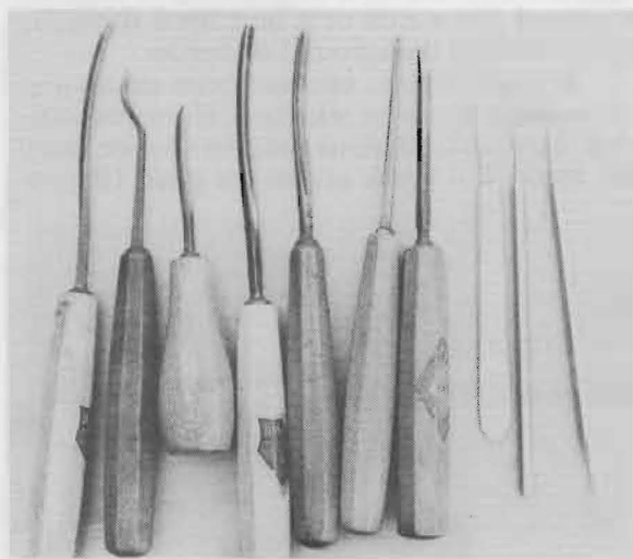
FIGURE 42 — Representative tools used by Colonel Miller for wood carving. Note surgeon's scalpel third from right.
