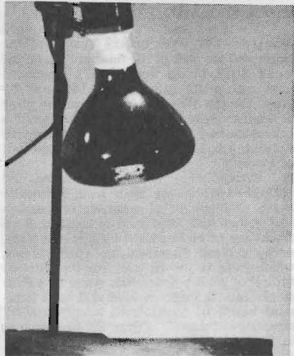
FIGURE 32 — An infrared lamp can be used to boil out the oil from blackened, oil saturated stocks. It never completely dries. (Photo courtesy NRA)
