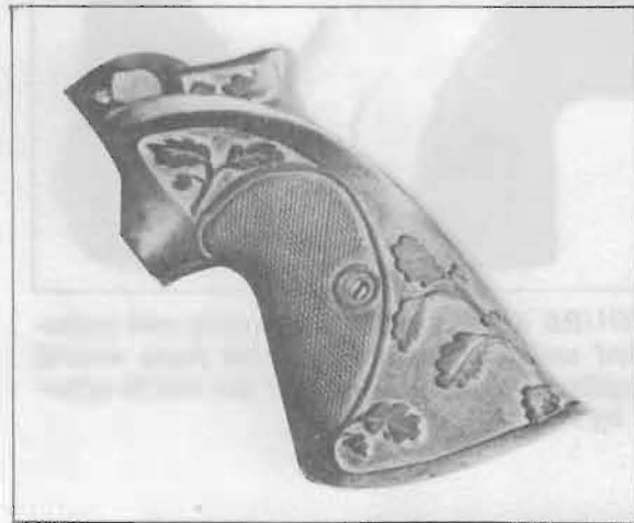
FIGURE 63 — Checkering, carving, and stippling are more often used to fancy-up a handgun stock than are "exotic" grains.
