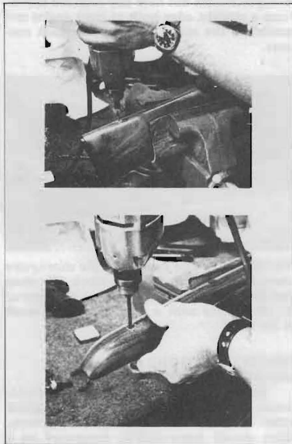
FIGURE 28 — Holes for sling swivels can be drilled after the stock is finished. It's better to do the job before the finish is applied, to prevent splintering around the holes.
