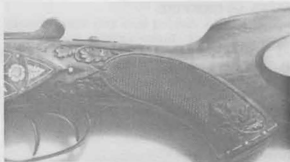
FIGURE 30 — Floral carving is often combined with checkering. The carving is always done first.
