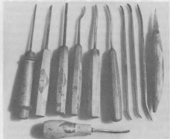
FIGURE 31 — Typical tools used by the advanced carver. However, a sharp knife and a few chisels are all you need to get started.
