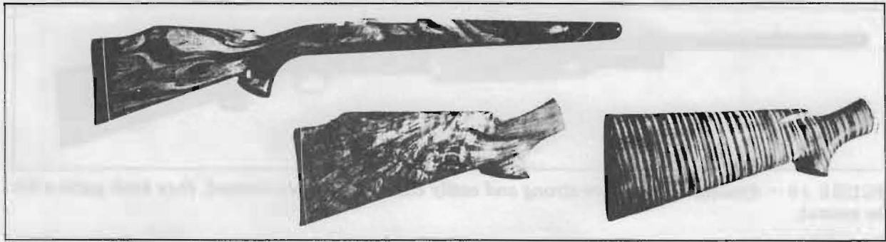
FIGURE 16 — Three distinctive domestic stock woods: top, screwbean mesquite; bottom left, black walnut, crotch; bottom right, black walnut, fiddleback. (Photos courtesy National Rifle Association)
