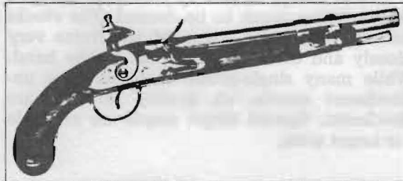
FIGURE 54 — Early pistols, like the flintlock U.S. Army model of 1818, had one-piece stocks with inletted sideplates. (Photo courtesy Small Arms of the World, Stackpole Book Co.)
