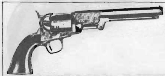
FIGURE 55 — Early Colts, like the Navy model of 1851, had a one-piece wood stock. (Photo courtesy Small Arms of the World, Stackpole Book Co.)
