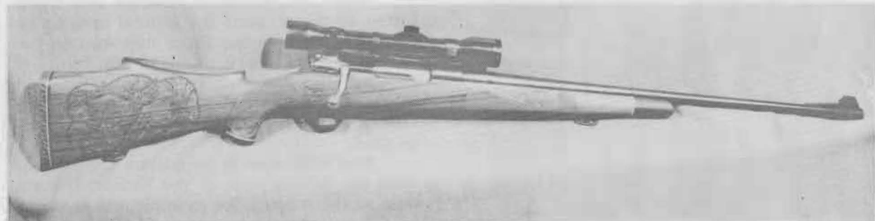
FIGURE 39 — A fine example by a master craftsman: a Mauser sporter embodying a carved stag and background, floral design and scrollwork, and fine 28-line checkering. From the collection of Colonel Miller.
