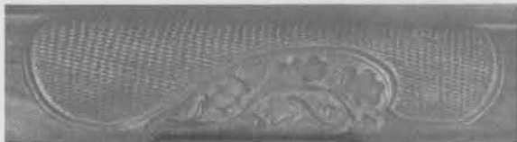
FIGURE 27 — Stippling is often used in combination with carving and checkering. In the above pattern, stippling was used to break the leaves away from the background.
