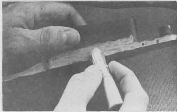
FIGURE 7 — Lipstick works as well as Prussian blue for "spotting." Here, it's being applied to the sides of the magazine and the floor plate.
