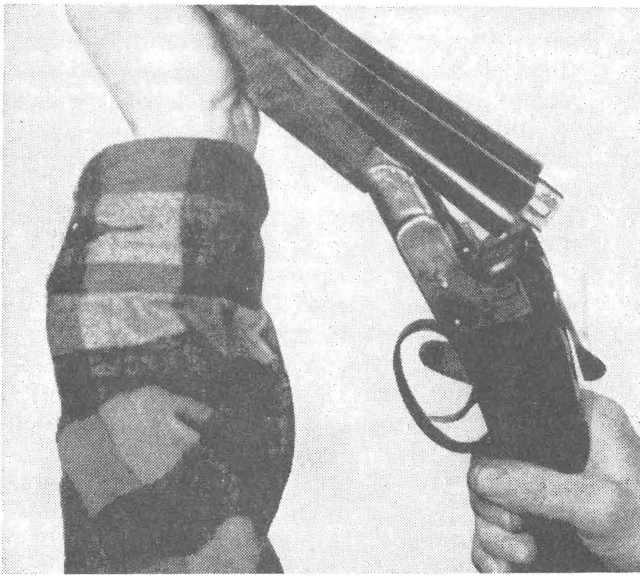
FIGURE 15 — Excessive “play” in an action usually means the gun is badly worn. Double shotguns (left) are checked by opening the action and twisting. Bolt-actions are checked with the bolt open and then closed, by twisting and jiggling the cocking piece and the bolt. Sometimes a badly worn cocked rifle will “fire” when the cocking piece is twisted. Excess wear, with a bit of practice, is easily detected.
