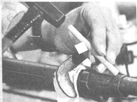
FIGURE 20 — Old barrel bands can be tough to remove. Plenty of penetrating oil, a C clamp to compress the band retainers, and a wooden dowel tapped with a hammer usually do the job.
