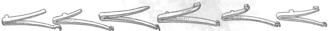
FIGURE 15 — Types of mainsprings used in the various makes of muzzleloading rifles and shotguns. The similarities are pronounced, but sufficient difference remains to make interchangeability impossible.
