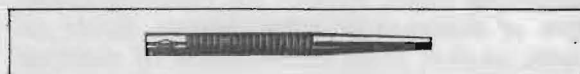
FIGURE 12b — Always use starting punches to break loose stuck or tight pins to protect both the pin punch and the gun. These starting punches are designed to start the most rusted or frozen pins. (Drawing courtesy Brownells, Inc.)
