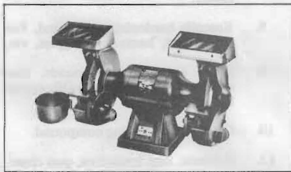
FIGURE 19 — A bench grinder is not essential in your gun shop, but it's nice to have and useful for working on both metal and wood.
