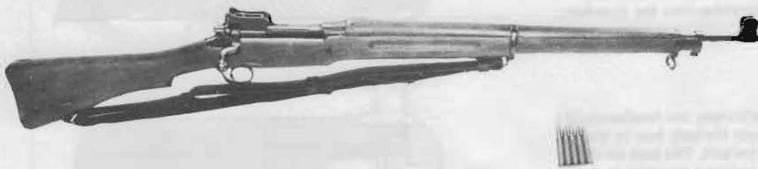
FIGURE 2 — This .30/06 caliber Enfield was often called the "British Springfield." Originally chambered for the .303 British, it was manufactured in .30/06 caliber during World War I. The Enfield has a long action and is suitable for magnum conversions. (Reprinted from Small Arms of the World, courtesy Stackpole Book Co.)
