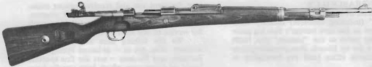
FIGURE 3 — The 98K German Mauser 7.92mm incorporates the famed Mauser 98 action, which is used today with only slight modifications on many contemporary custom sporters. (Reprinted from Small Arms of the World , courtesy Stackpole Book Co.)
