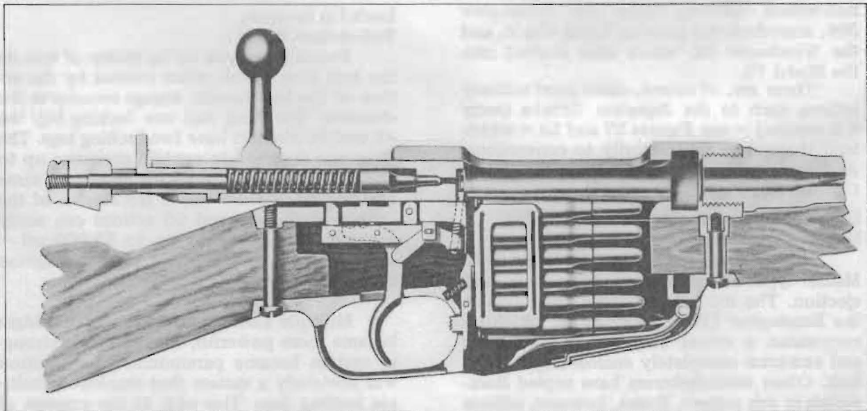
FIGURE 30 — Carcano cutaway view showing the action open and with loaded clip magazine. This firearm cocks on closing like the early Mausers.
