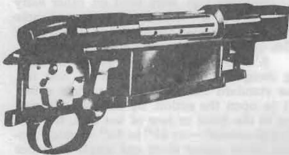
FIGURE 34 — Weatherby Mark V, showing triple gas ports in the side of the bolt.
