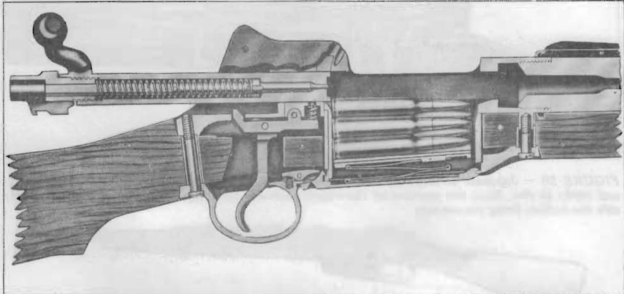
FIGURE 26 — U.S. Model 1917 Enfield (Pattern 17), one of the simplest and strongest bolt-action rifles ever made. Cutaway shows the bolt open, ready to move forward and strip the top cartridge from the magazine.
