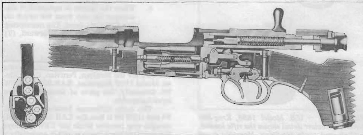
FIGURE 21 — Mannlicher-Schoenauer European sporting rifle with double-set triggers. Spool-type magazine served as "inspiration" for the first Savage lever-action, the Model 1895.
