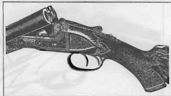
FIGURE 36 — Parker shotgun, one of the most valuable of all American vintage doubles, and a prime example of the doll's head lock-up system.
