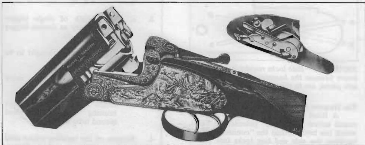
FIGURE 26 — Back-action side locks have all lock components mounted to the rear of the side plate, with the mainspring positioned behind the hammer. The gun shown is the AYA M37, a super-deluxe Spanish double.
