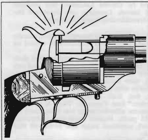
FIGURE 3 — The Lefauchaux pin-fire ignition system was widely used in pistols as well as in shotguns and rifles. The above cutaway drawing shows the priming system as used on an early revolver.
