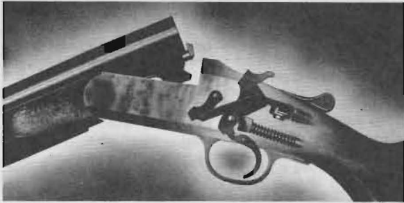
FIGURE 8 — The small number of parts and simplicity of design inherent in the single-barrel action are shown in this cutaway of the Stevens M94 exposed-hammer shotgun.
