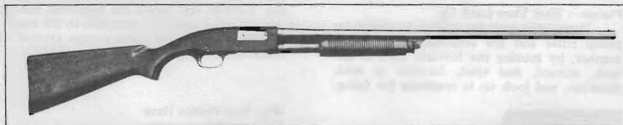
FIGURE 44 — The Remington Model 31 had a remarkably smooth action, and ejected shells out the side.
