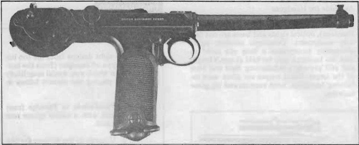
FIGURE 13—The first successful auto-pistol was the American-designed but German-manufactured Borchardt, first produced in 1893. It used a bottleneck cartridge very similar to the modern 7.63mm Mauser pistol cartridge.
