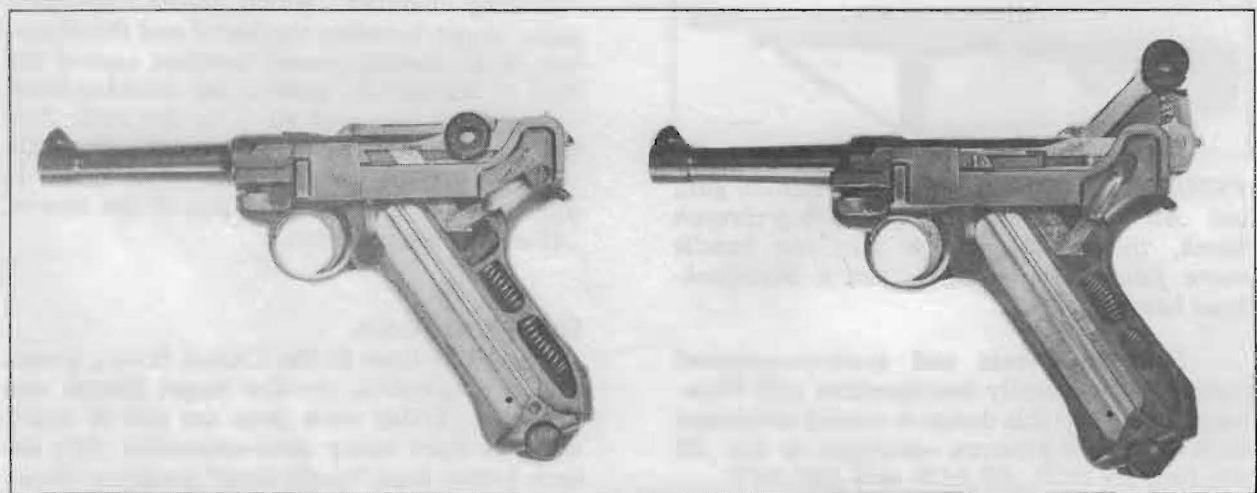
FIGURE 17 — Cutaway views of the famous Luger pistol. Drawing to the left shows the action closed. The righthand drawing shows the action open, with toggle raised. Note the different positions of the recoil spring hook-up in the rear of the grip.
