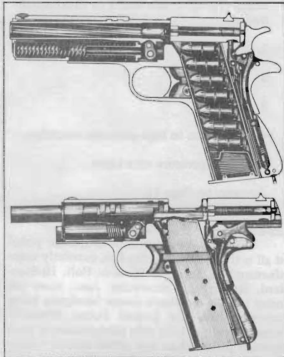
FIGURE 16 — Details of the locking and firing mechanisms for the Colt 1911A1. The top drawing shows the action closed with the pivoting barrel link at rest. The bottom drawing reveals the details when the action is open and cocked. Note how the barrel has swung back and down on the pivot link during unlocking.
