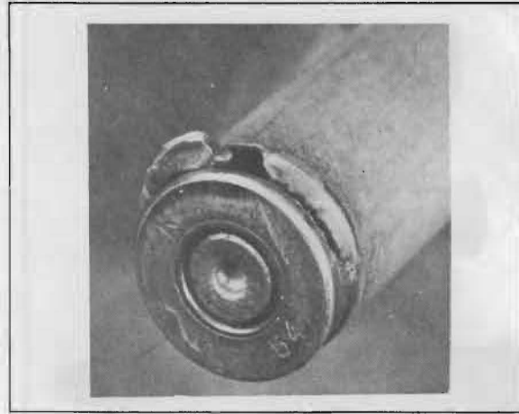
FIGURE 24 — Flaws in cartridge case manufacture are fairly commonplace, especially with military ammo where the quality control isn't as rigid as for sporting ammunition. The case rupture shown resulted from too much hardening alloy in the metal "mix."
