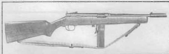
FIGURE 19 — The Reising submachine gun, cal. .45 ACP. Because of its heavy breech block, this blowback-type gun can handle more powerful cartridges than a blowback-type handgun.
