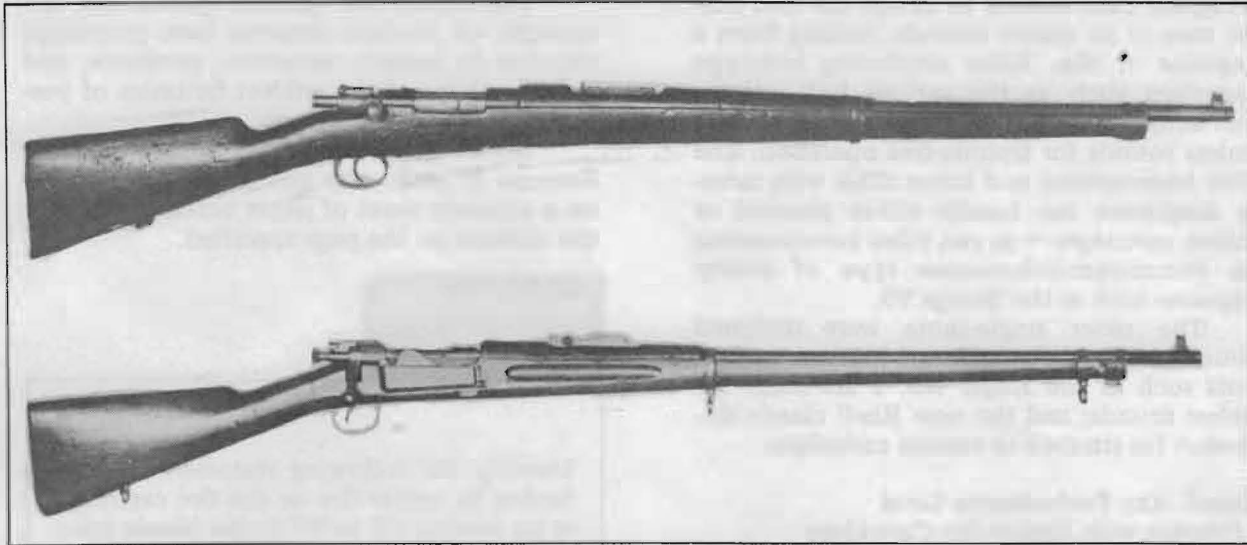
FIGURE 25 — The Spanish 7mm Mauser (top) was one of the first military rifles to use a rimless cartridge and staggered-column magazine. The contemporary U.S. Krag-Jorgensen service rifle (bottom) used the .30-40 rimmed cartridge and had an unsatisfactory box-type magazine. Both rifles were used in the Spanish-American War.
