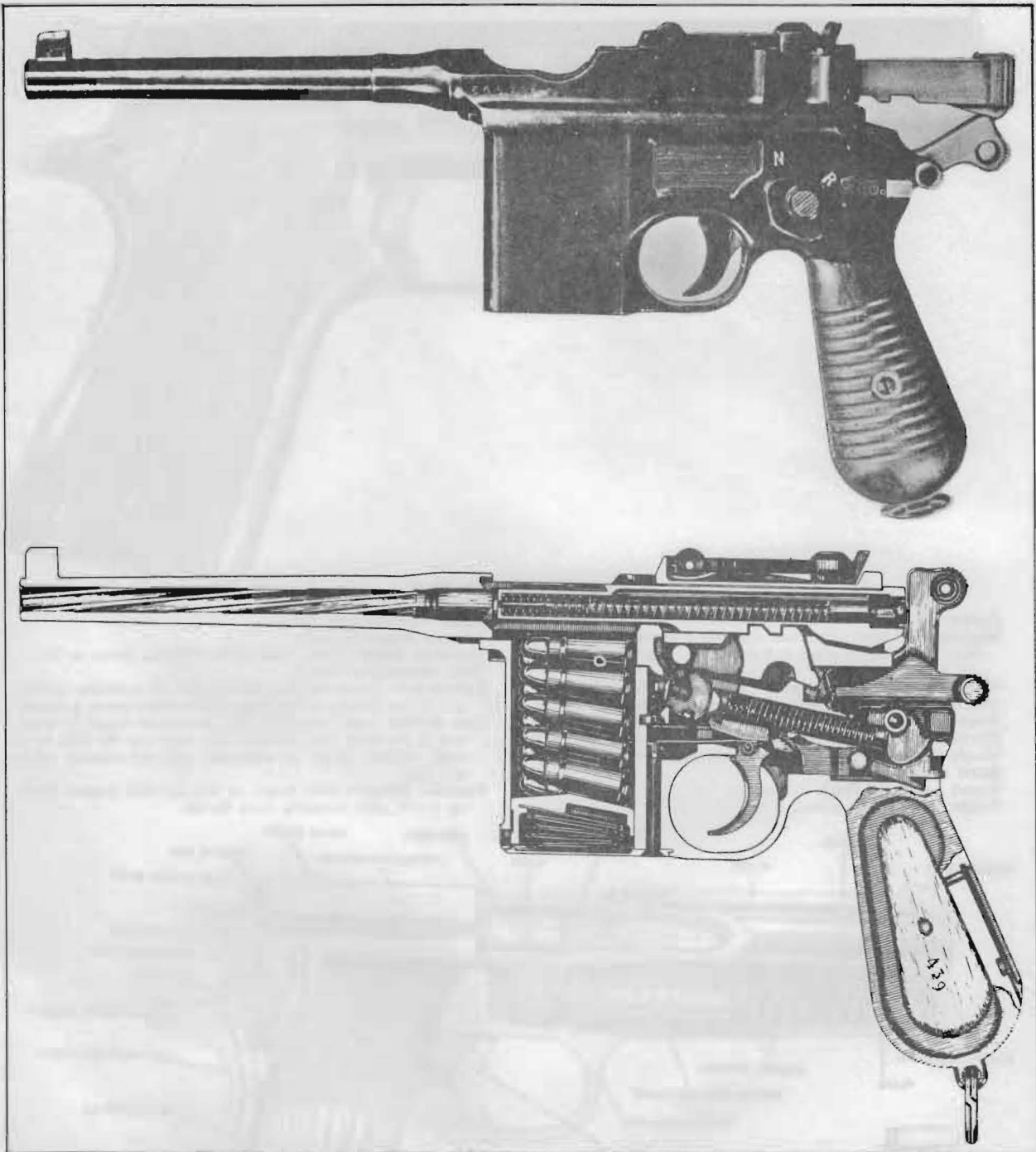
FIGURE 14 — An early Mauser military pistol chambered for 7.63mm and 9mm Mauser and 9mm Luger cartridges. Note that the magazine is positioned forward of the trigger, not in the butt like modern auto-pistols. Cutaway photo shows details of Mauser mechanism and magazine, action closed.
