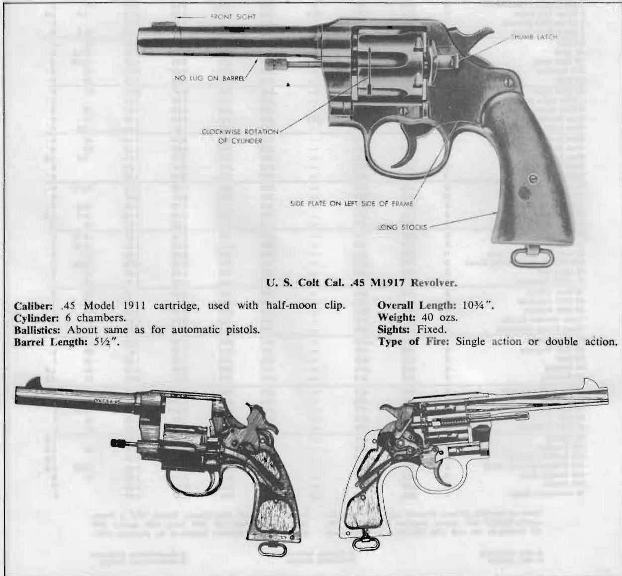
FIGURE 33 — The Colt M1917 service revolver, which was chambered for a rimmed version of the .45 Colt ACP rimless cartridge. The latter could be fired in the gun with the use of half-moon clips. Cutaway at left shows position of mainspring with hammer cocked and cylinder swung out. Right-hand drawing shows detail with all parts at rest.
