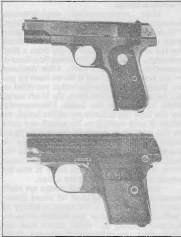
FIGURE 18 — The Colt .25 Pocket Auto (top) and its big brother, chambered for the .32 and .380 ACP cartridges, are examples of blowback design, suitable only for relatively low-pressure cartridges.
