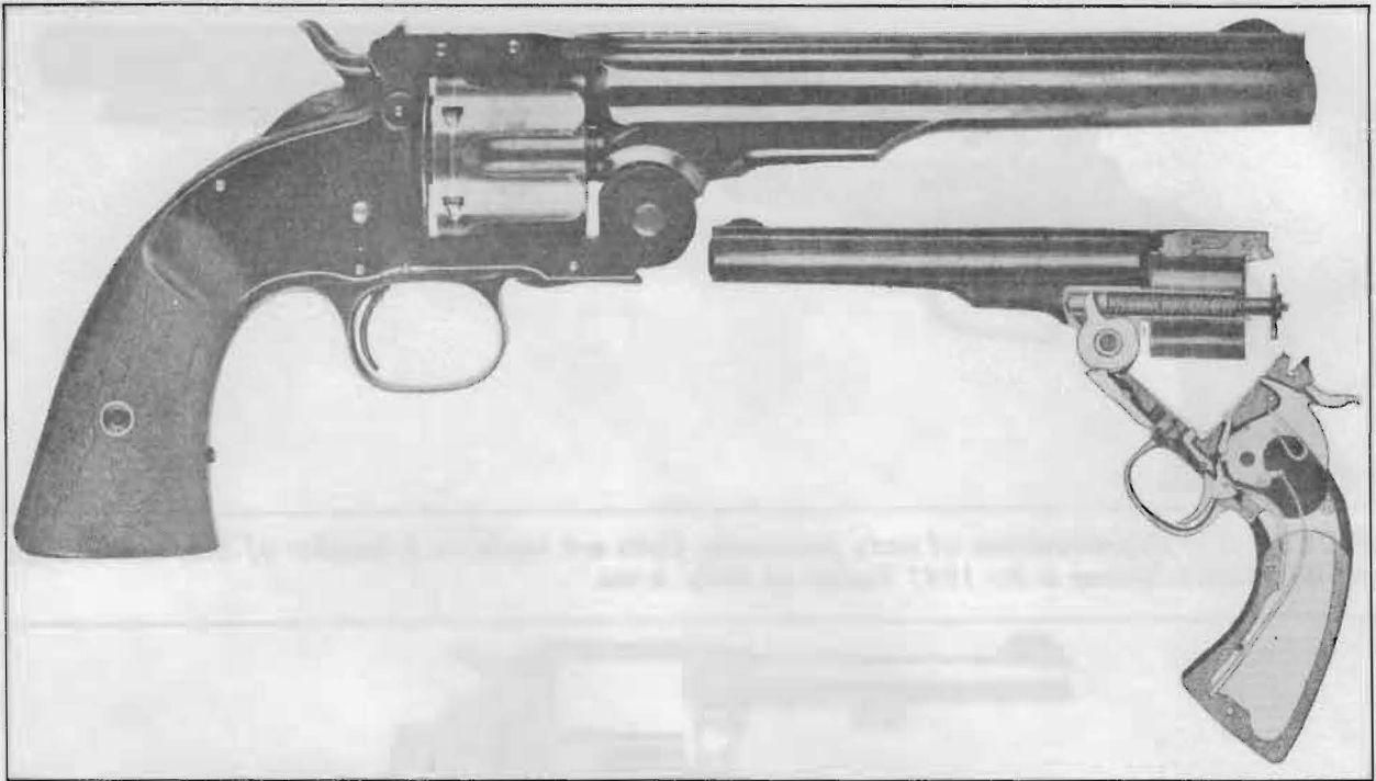
FIGURE 6 — Early S&W Schofield, Model 1875, illustrates typical “tip-up” revolver design. The cylinder doesn’t flip out, but is exposed for rear loading. This .45-caliber single-action six-shot was one of the strongest hinged-frame revolvers ever built.
