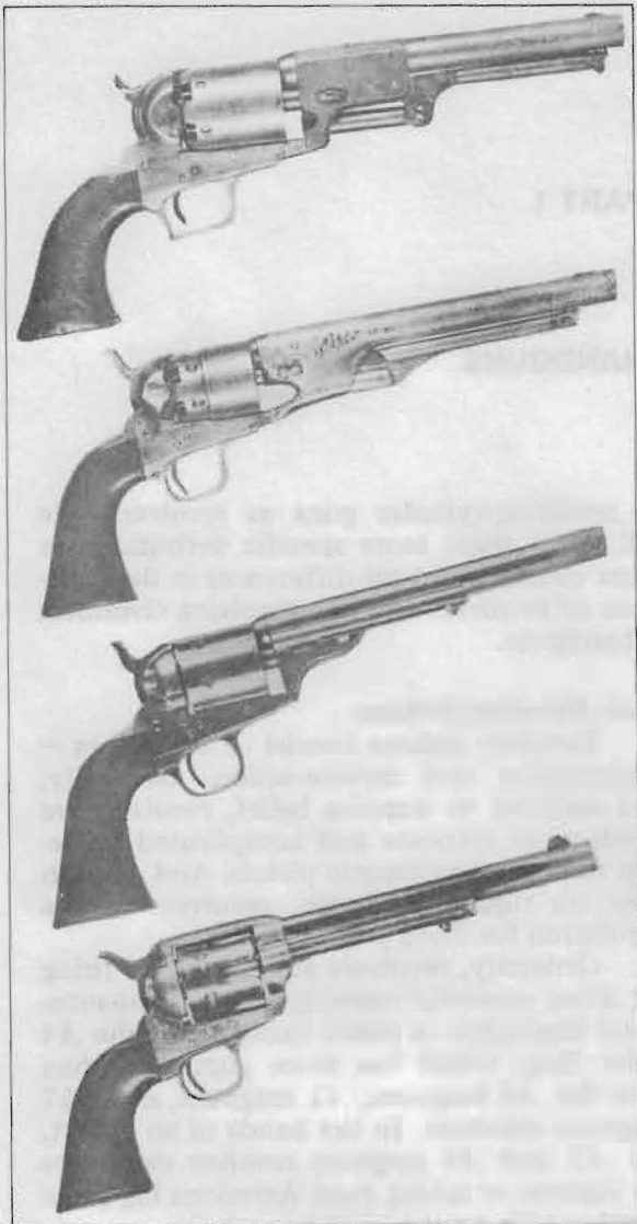
FIGURE 2 — The early Colt revolvers, all single-action "six-shooters." From top: the Dragoon model of 1848, .44 cal., percussion-primed; the "New Army" model of 1860, principal revolver of the Civil War, .44 cal., percussion-primed; the Model 1872, the first Colt to fire metallic cartridges, .45 cal.; Colt Model 1873, first solid-frame Colt and the most popular ever produced. It was made for 70 years with few or no changes.
