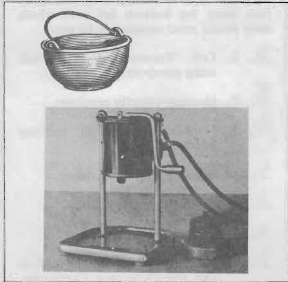
FIGURE 10 — Before casting bullets, the lead must be melted — in a container as simple as the old Ideal pot offered by Lyman (top) or as “advanced” as the Potter Electric Furnace (bottom).
