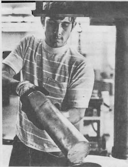
FIGURE 21 — A craftsman at Sierra Bullets inserts a heavy lead alloy billet into an extrusion press which forms lead "wire" used in core manufacturing.
