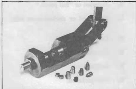
FIGURE 11 — The Herter 9-Ton Bullet Maker uses adjustable dies to swage jacketed or lead alloy bullets in a variety of nose shapes.
