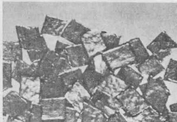
FIGURE 16 — The first smokeless powder was of the flake variety, similar in appearance to Rottwell No. 5, shown above. As fire-retardant coatings weren't yet invented, the flakes burned too fast for the guns of the period.
