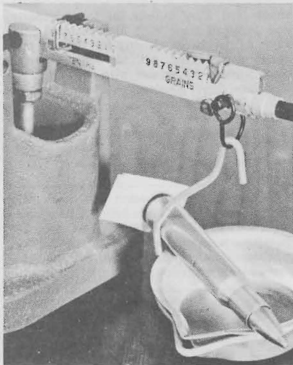
FIGURE 4 — To determine case capacity, first weigh the case with the bullet seated to the proper depth. Affix a bit of tape over the base. After getting this weight figure, fill the case with water and weigh it again. (The tape keeps the water from leaking out.) (Photo courtesy "Handloader Magazine")
