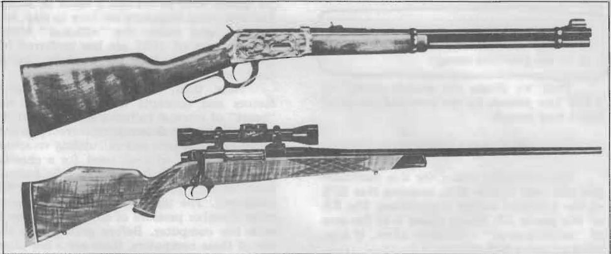
FIGURE 18 — It is virtually impossible to shoot out the barrel of an oldtimer like the Winchester Model 94 .30/30 at the top. A newer gun, like the Weatherby, can be shot out in 1,000 rounds or less if the barrel isn't allowed to cool between rounds.
