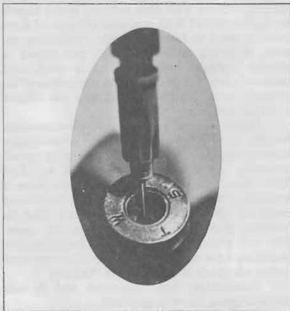
FIGURE 5 — The best way to fill a case is with a hypodermic needle. Fill the case slowly through its flashhole. When the hypo is empty, it can be used to blow out the water from the case, permitting two or three measurements for an average.
