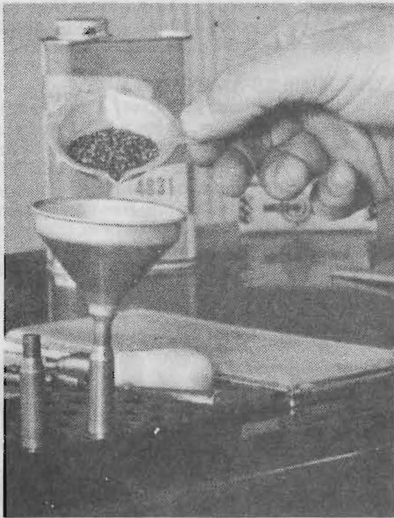
FIGURE 17 — When your case gets so full you have to use a funnel and “tamping” to fit the charge into the case, it’s time to change to a smaller quantity of a faster-burning powder.
