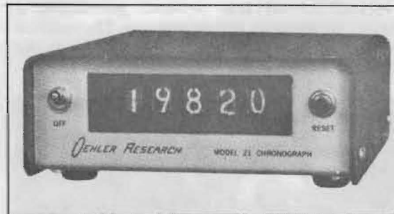
FIGURE 8 — Digital chronographs like the Oehler Model 21 are relatively expensive, but provide a direct read-out of velocity.
