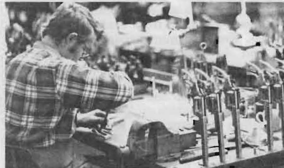
FIGURE 27 — Threaded and in-the-white barrels are first rough-fitted, as shown in this S&W factory photograph. They will later be checked for headspace and polished prior to bluing.
